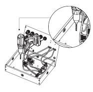
Mark and drill out the mounting holes for mounting the control box on the wall. Make sure to clean out all the aluminium swarf created from drilling.
