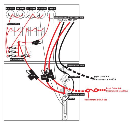
+ Once complete, the LED display on the voltmeter should be an indication of power going into the panel. If there is no power, check cabling, wiring, 12v switch is on, test using a 12v multimeter, or contact a licensed auto electrician.
