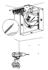
Lift the control box onto desired location, mark the locations of the drilled mounting holes on the canopy wall. Remove the box and drill the holes accordingly.
